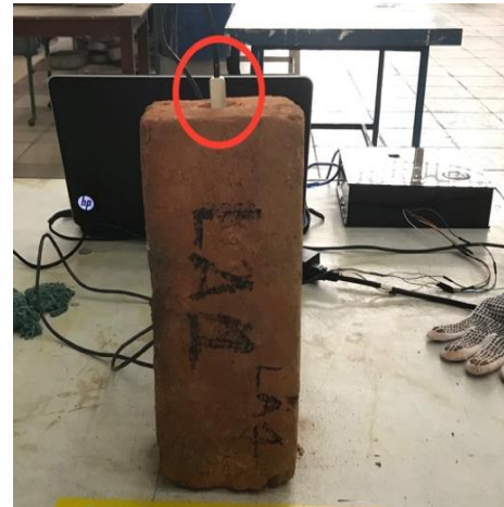
Figure 5. Thermal needle probe on a block of cooked clay
