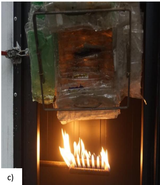
Figure 2 Photographs that show testing of combustibility and optical density of recycled PET bottles. a) Lattice of metal rods for the manufacture of the test tube, b) arrangement of the PET sheets extracted from the bottles to be able to form the test tube, c) detail of the burners located in the lower part of the test tube. Source: Own elaboration.
